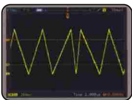
Slope trigger Ascertain trigger time neatly by signal slew rate
